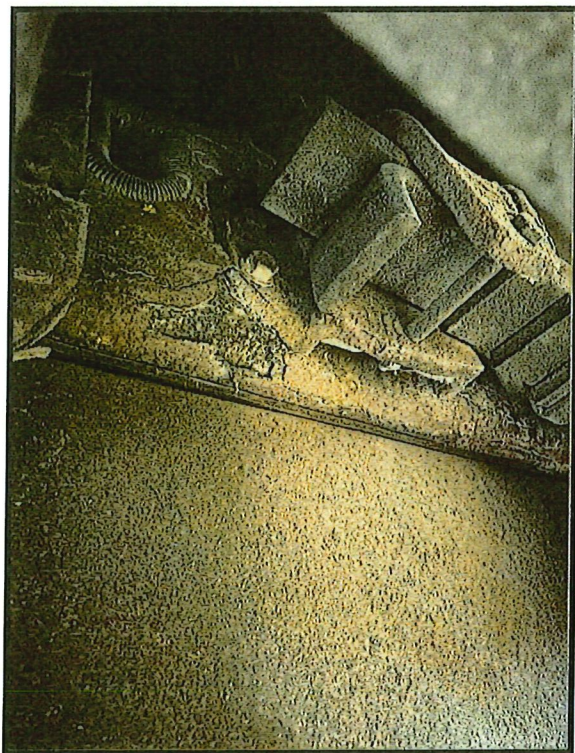
Drivers Side Rear Spring Perch Mount Showing Delamination
