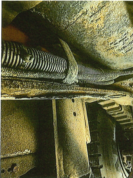
Passenger Side Inner Frame Rail Showing Delamination
