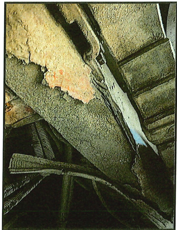
Drivers Side Frame Rail Showing Extreme Delamination
