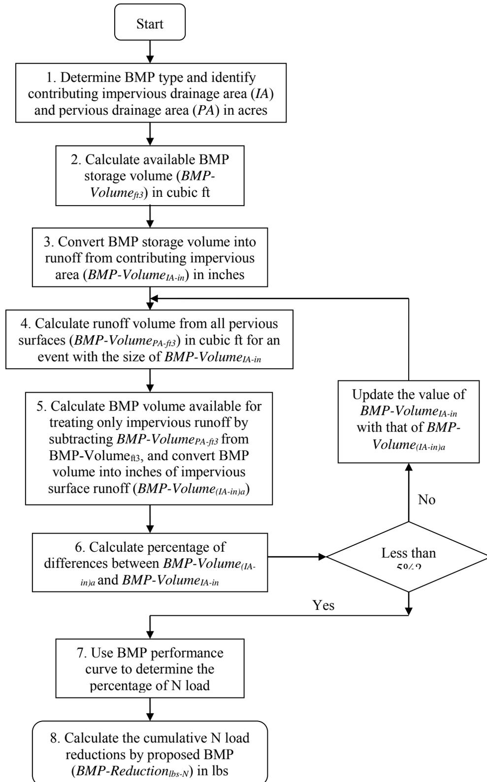
**Flow Chart 2 (previous page). Method to determine the nitrogen load reduction for a BMP with known storage volume when both pervious and impervious drainage areas are present.**
