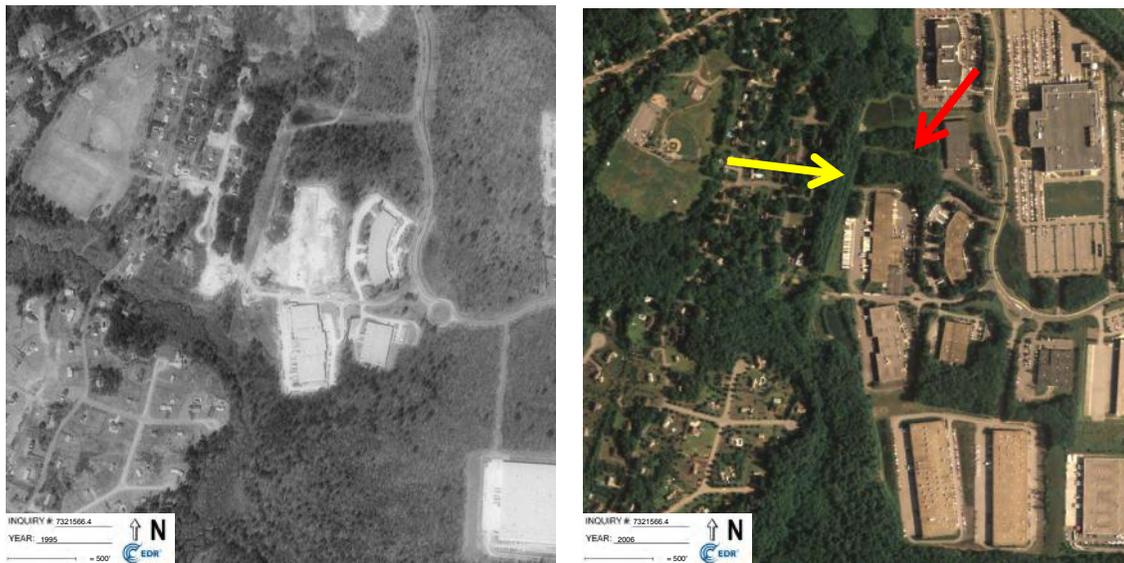
Figure 5: Side-by-side historic aerials from 1995 and 2006. Tree clearing for drainage infrastructure is absent in 1995 imagery but visible in 2006 imagery. The offsite stormwater ditch (i.e. A- and F-series wetlands) is indicated in red. The location of the B-series IVW is indicated in yellow.
