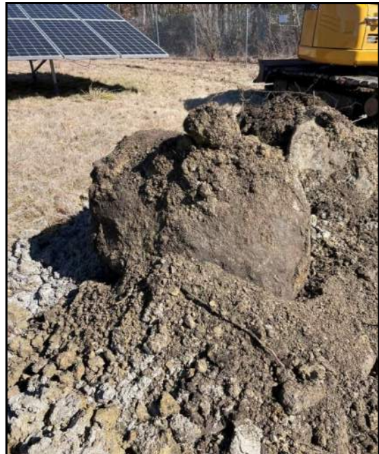
TP-116 spoils pile with large boulder
