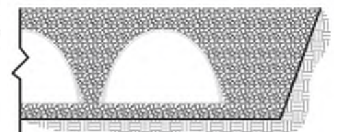
Perimeter Fully Backfilled
