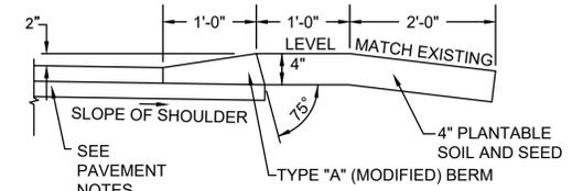
**HMA BERM - TYPE "A" (MODIFIED)
