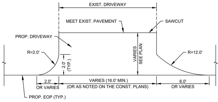
**DETAIL FOR DRIVEWAY WITHOUT SIDEWALK (W/O BERM)**
