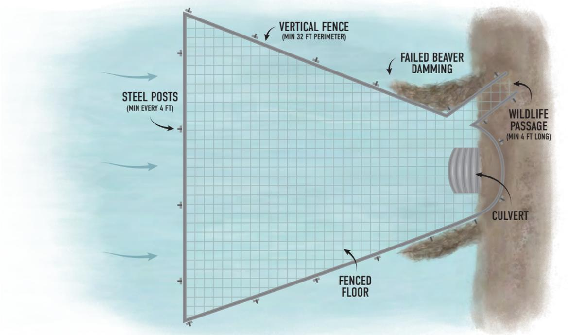
Figure 8. Trapezoidal culvert fence.
