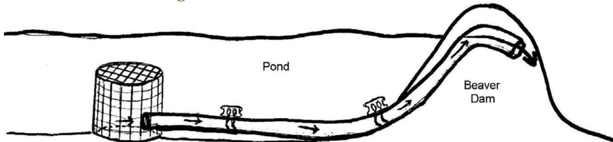
Created by Michel LeClair in Canada, the Flexible Pond Leveler pipe system works because the fencing on the pipe intake keeps the beavers far enough from the inlet so they do not feel or hear water flowing into the pipe. If the beavers cannot detect the flow of water into the pipe, they do not try to block it. The pipe is placed through a trench dug in the dam. The height of the pipe in the dam controls the pond level.
