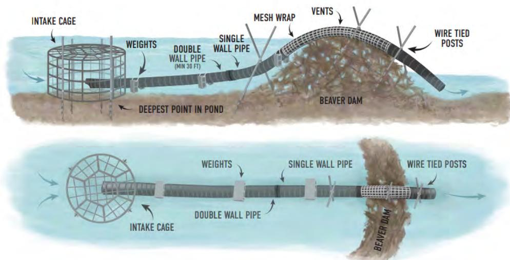
Figure 3. Standard pond lever design with no modifications (BeaverCoalition, 2022)
