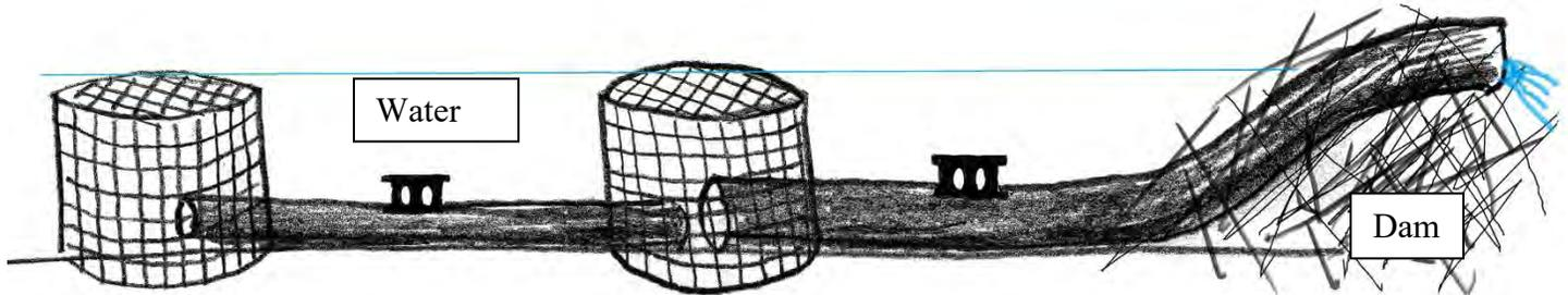
The “*Multi-Intake Leveler*” design is based on the highly successful *Flexible Pond Leveler™* which has been successful in thousands of locations. This pipe system is intended specifically for use in narrow channels or where there is inadequate depth for a standard *Flexible Pond Leveler*. See diagram.
