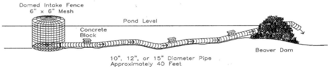
In order for these pipe systems to be effective, they must be designed so that beavers cannot detect the flow of water into the pipe. The Flexible Pond Leveler™ does this by surrounding the submerged intake of the pipe with a large cylinder of fencing which is placed in as deep water as possible. This prevents the beavers from detecting the flow of water into the pipe. As a result, the beavers do not try to clog the pipe, and a safe water level can be maintained.
