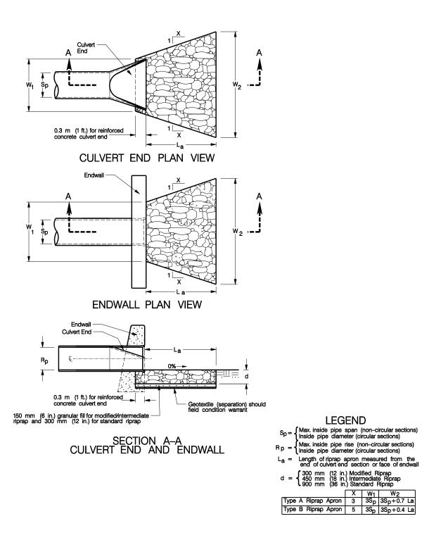
Figure 11-13 Type A and B Riprap Apron (to be used where there is no defined channel downstream of the outlet)
