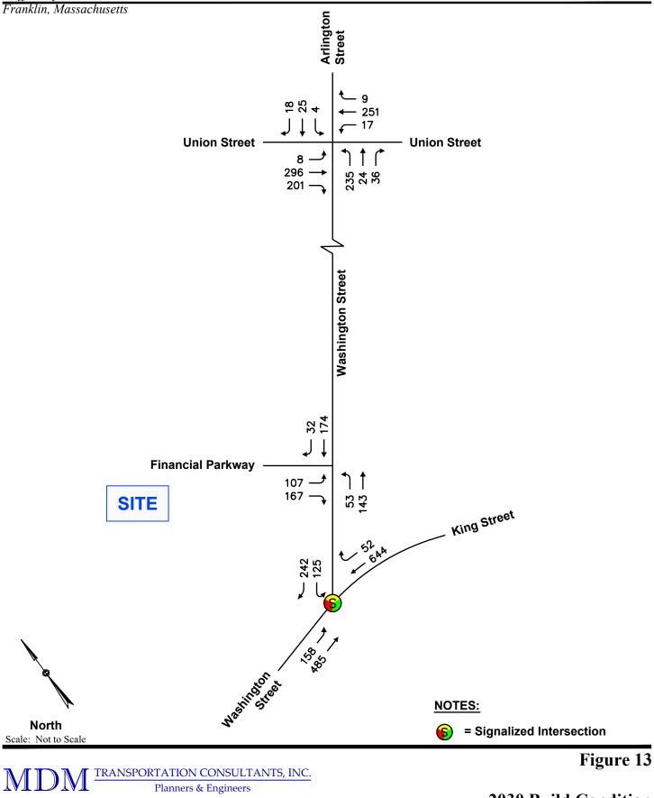
2030 Build Condition Weekday Afternoon Peak Hour Traffic Volumes Intersection capacity analyses are presented in this section for the Baseline, No-Build, and Build traffic-volume conditions. Capacity analyses, conducted in accordance with EEA/MassDOT guidelines, provide an index of how well the roadway facilities serve the traffic demands placed upon them.
