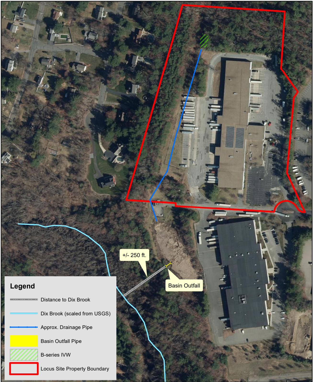
Figure 3: Orthophoto of site showing approximate location of +/- 1,000 linear feet drainage pipe extending from B-series stormwater IVW to southern offsite detention pond, and outfall from offsite detention basin.
