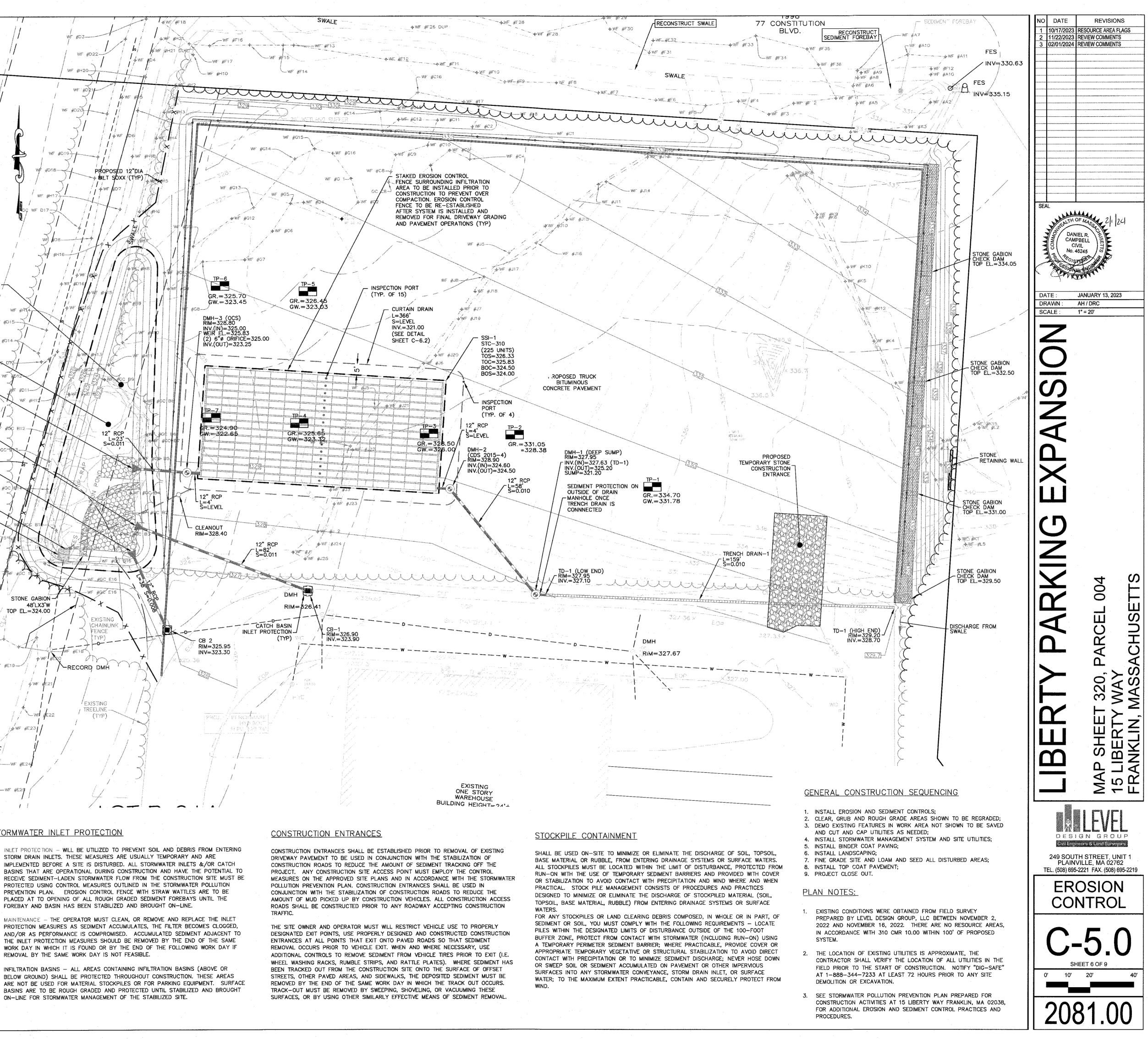
INLET PROTECTION - WILL BE UTILIZED TO PREVENT SOIL AND DEBRIS FROM ENTERING STORM DRAIN INLETS. THESE MEASURES ARE USUALLY TEMPORARY AND ARE IMPLEMENTED BEFORE A SITE IS DISTURBED. ALL STORMWATER INLETS &/OR CATCH PROTECTED USING CONTROL MEASURES OUTLINED IN THE STORMWATER POLLUTION PREVENTION PLAN. EROSION CONTROL FENCE WITH STRAW WATTLES ARE TO BE PLACED AT TO OPENING OF ALL ROUGH GRADED SEDIMENT FOREBAYS UNTIL THE FOREBAY AND BASIN HAS BEEN STABILIZED AND BROUGHT ON-LINE.
