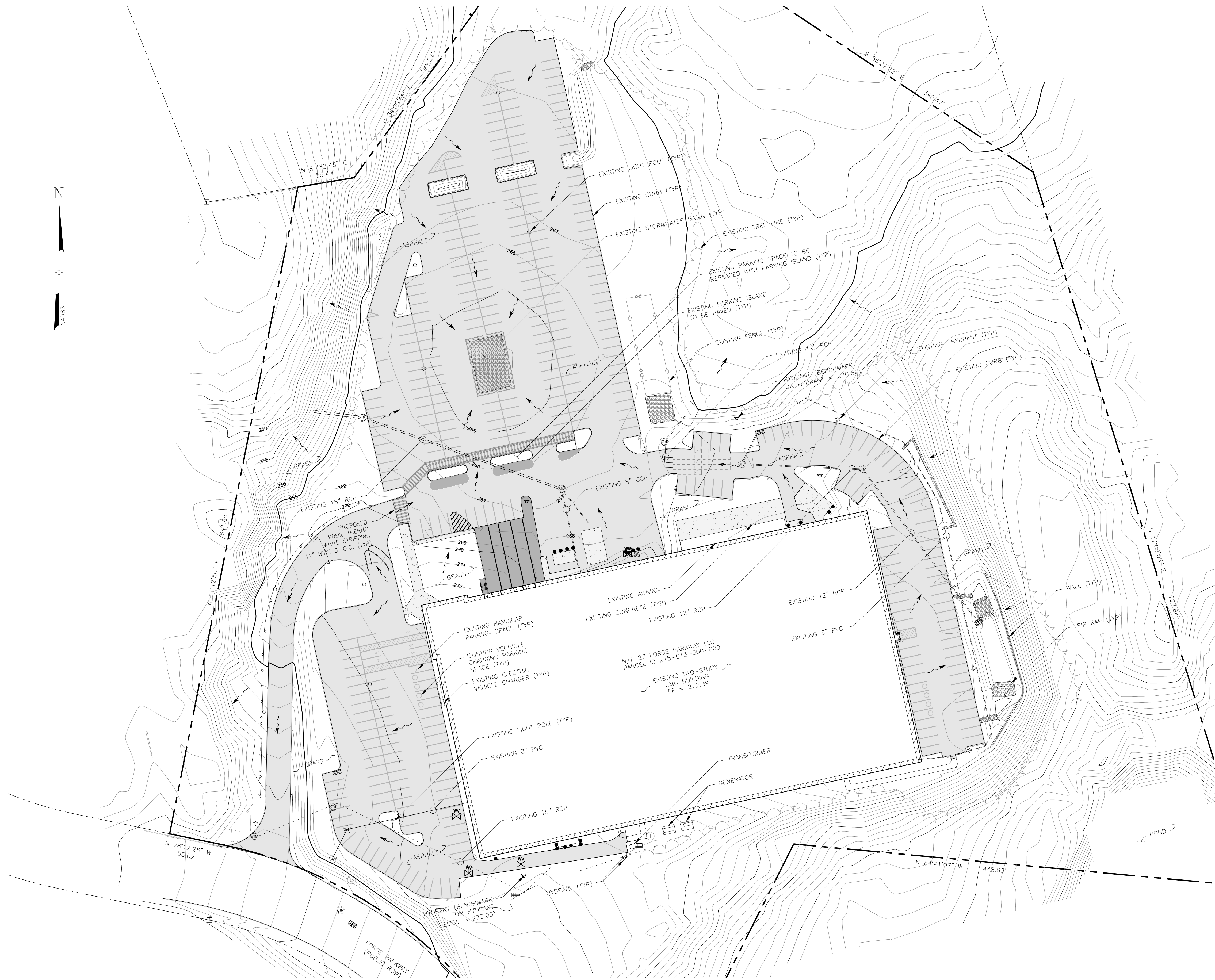
OVERALL DRAINAGE & GRADING PLAN
