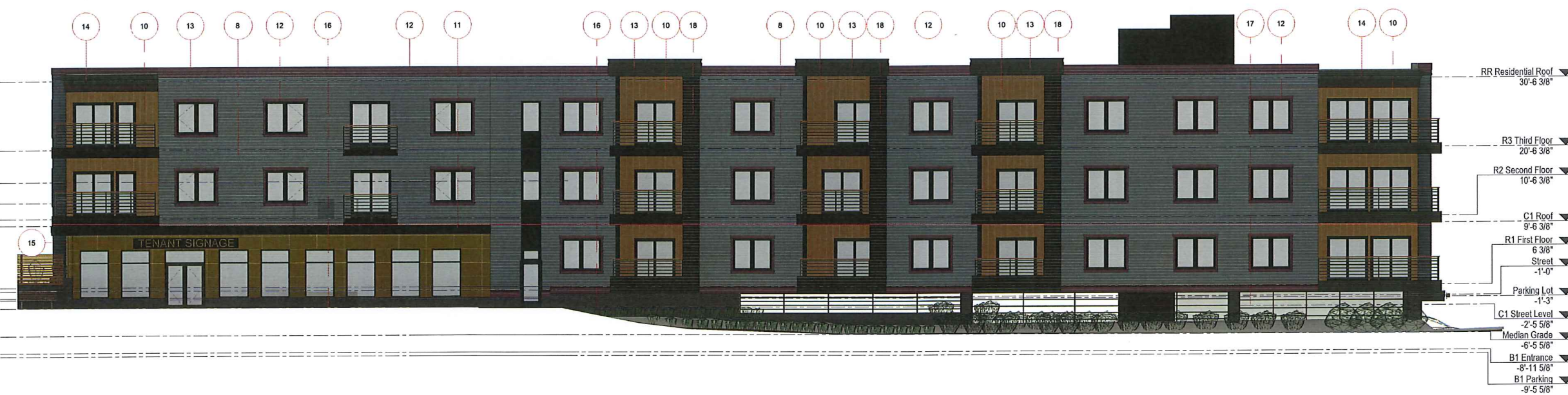
1 PROPOSED ELEVATION SOUTH A - STRUCTURE B A202 1/8" = 1'-0"
