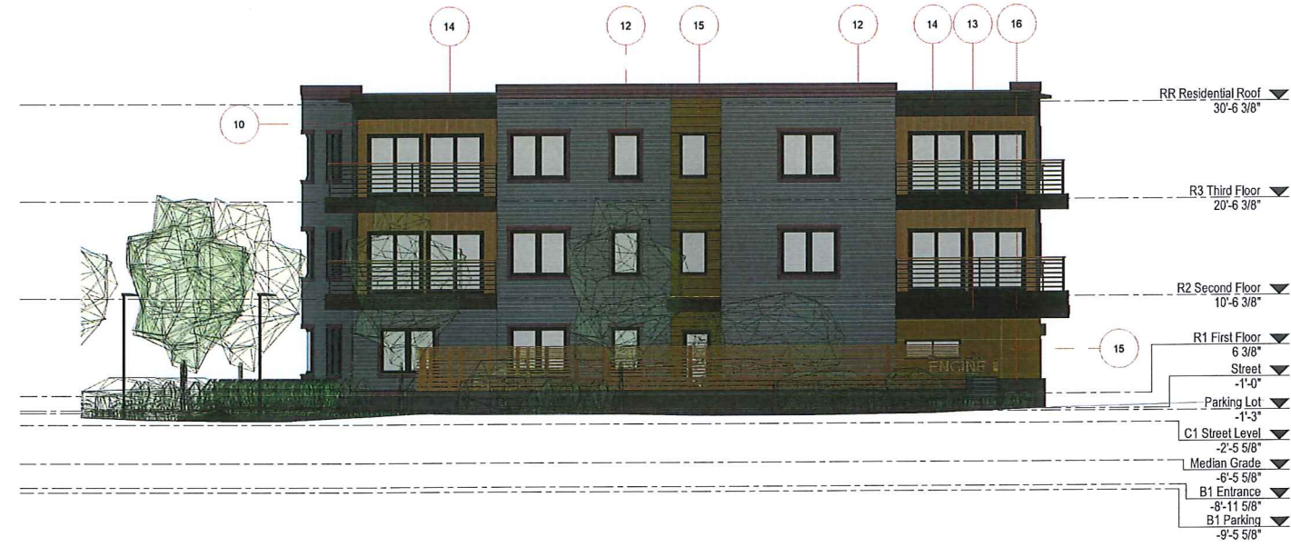
3 A202 PROPOSED ELEVATION WEST - STRUCTURE B 1/8" = 1'-0"
