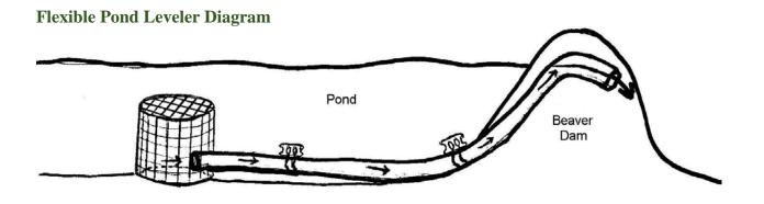
Created by Michel LeClair in Canada, the Flexible Pond Leveler pipe system works because the fencing on the pipe intake keeps the beavers far enough from the inlet so they do not feel or hear water flowing into the pipe. If the beavers cannot detect the flow of water into the pipe, they do not try to block it. The pipe is placed through a trench dug in the dam. The height of the pipe in the dam controls the pond level.
