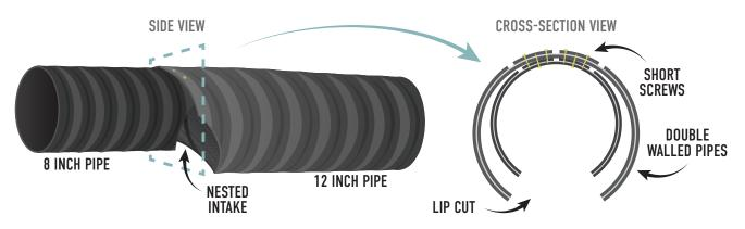
Figure 4. Nested pipe configuration used when constructing a dual-intake pond leveler.
