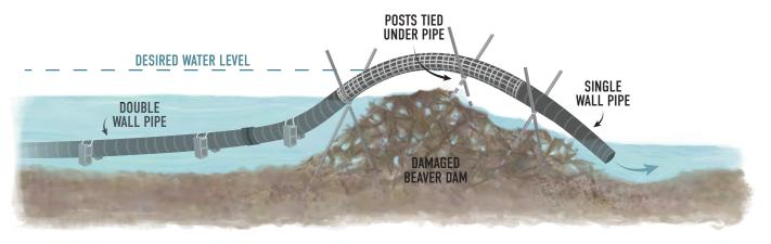
Figure 7. Installing or adjusting pond leveler to account for dam damage.
