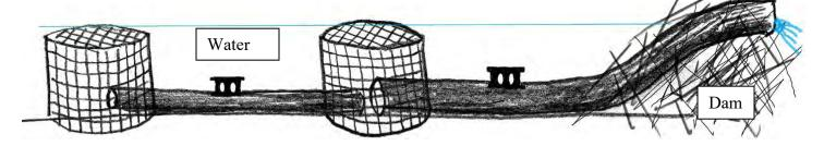
The "Multi-Intake Leveler" design is based on the highly successful Flexible Pond Leveler™ which has been successful in thousands of locations. This pipe system is intended specifically for use in narrow channels or where there is inadequate depth for a standard Flexible Pond Leveler. See diagram.
