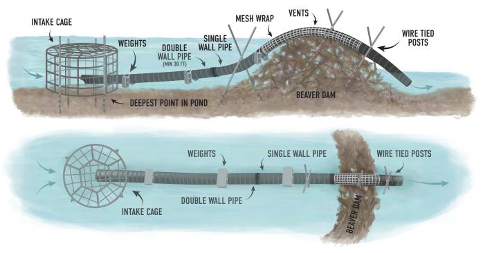
Figure 1. Standard pond leveler with no modifications.
