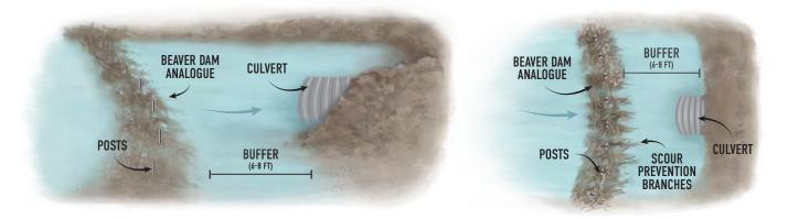
Figure 11. Anchor dam using a post-less BDA that is reinforced with steel posts.
