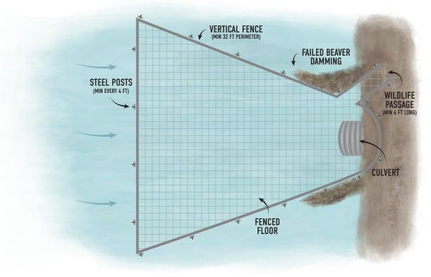
Figure 8. Trapezoidal culvert fence.
