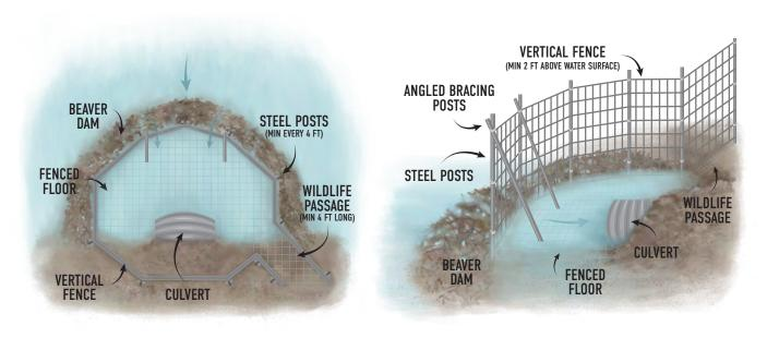
Figure 9. Standard anchor fence shown from above (left) and side (right)
