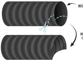
Figure 2. Modification to intake pipe and locations for pipe vent cuts.
