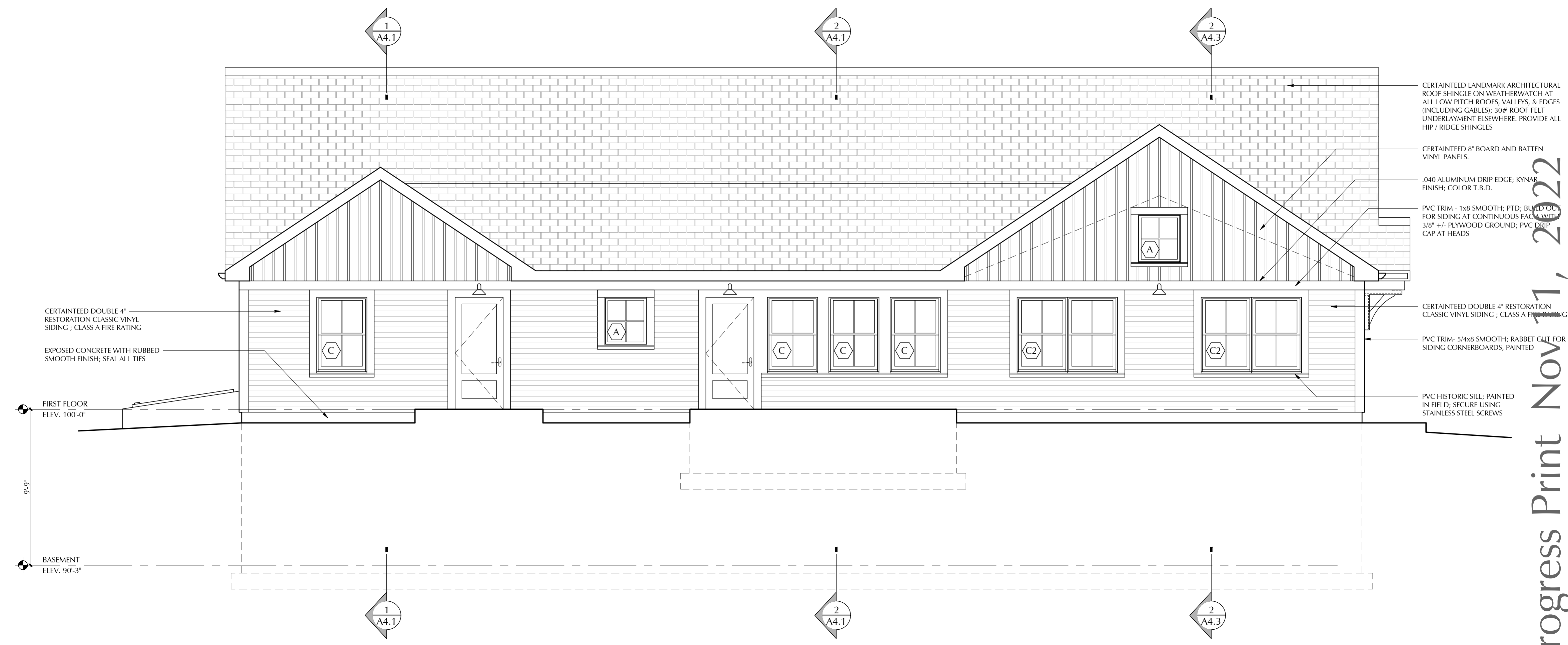
EXTERIOR ELEVATION - WEST SCALE 1/4" = 1'-0"
