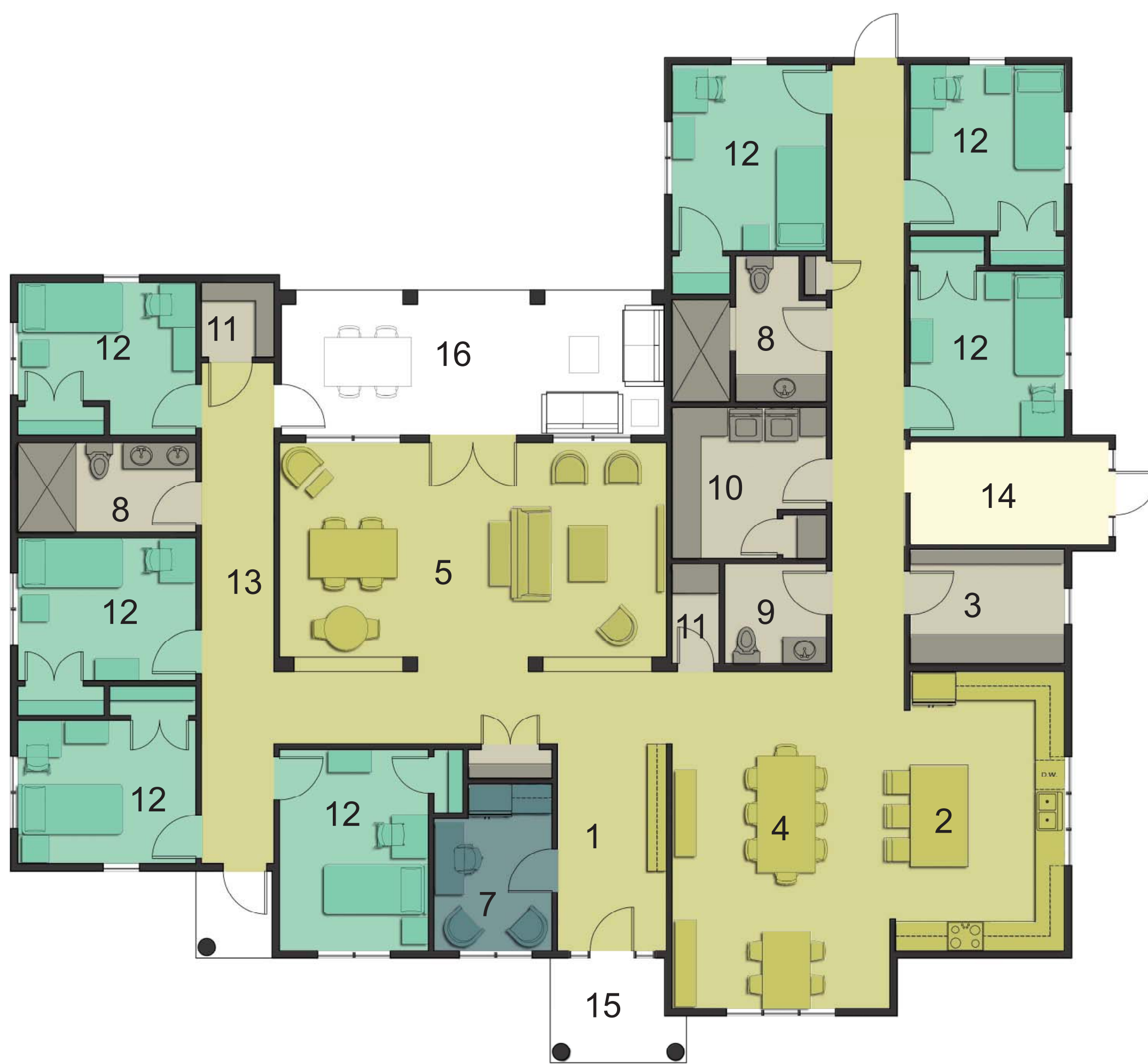
FLOOR PLAN - UNIT A SCALE: 1/8"=1'-0"
