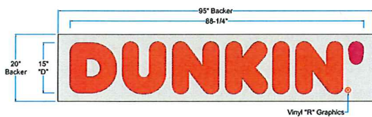
E1 Elevation: #12972.3 (Qty: 1) Face Illuminating Channel Letters Mounted to Backer Panel Channels 15' x 88.25' = 9.19 Sq. Ft. Backer 20' x 95' = 13.19 Sq. Ft.
