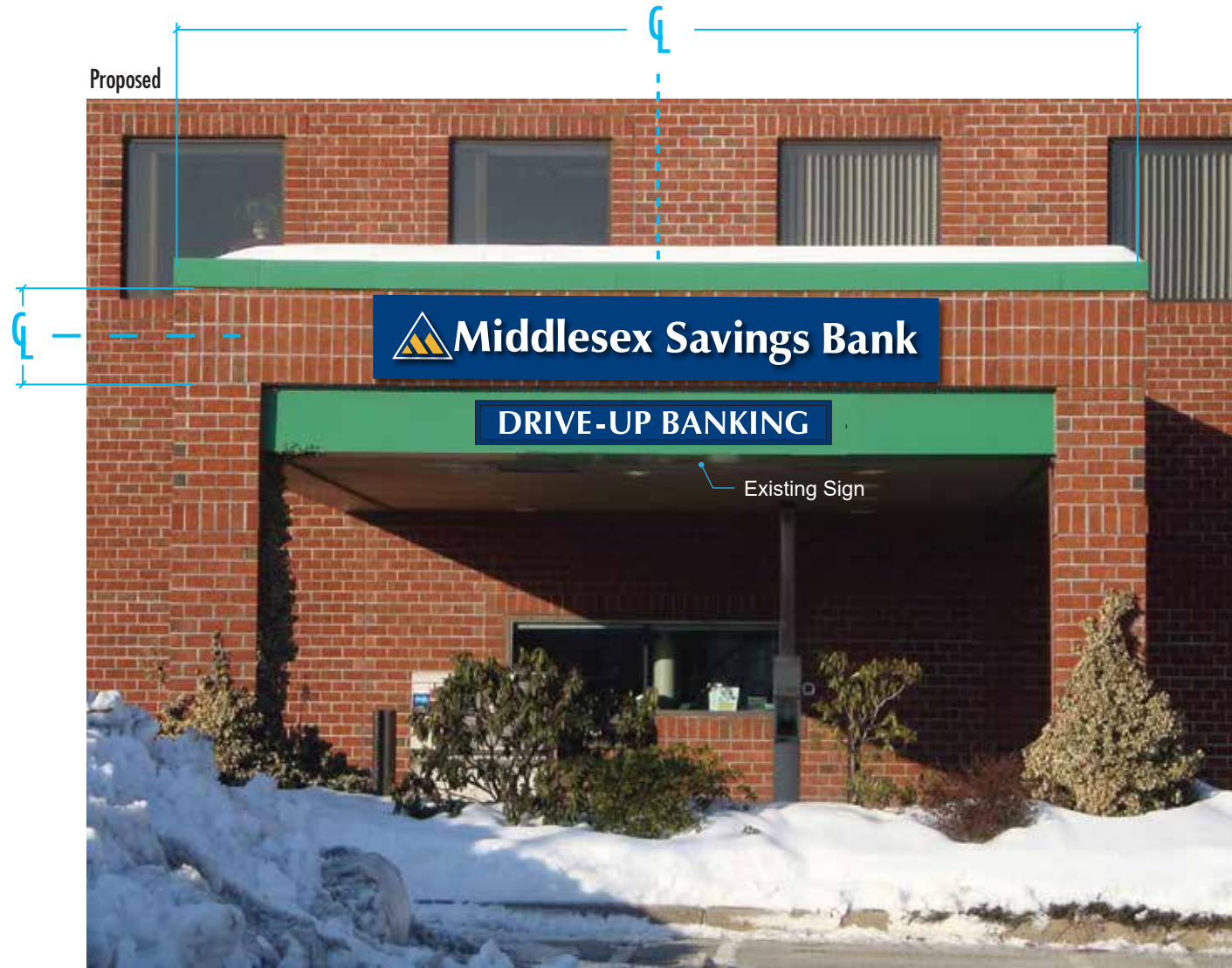
E2 Elevation: #12608.1 (Qty-1) Drive Thru Canopy Wall Sign Scale: 1/4"=1' Sq.Ft. 24"x162"=27 sf.
