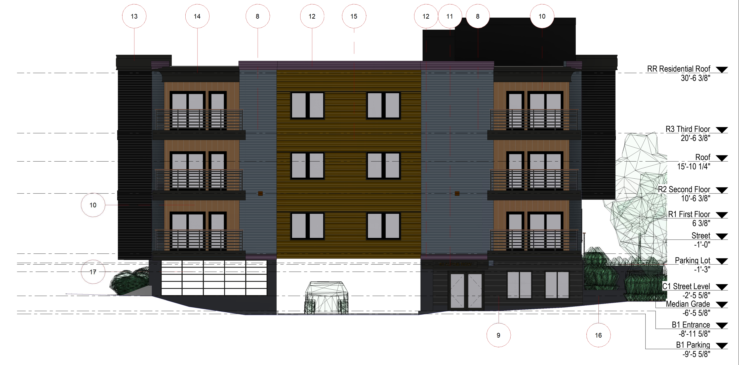
1 A201 PROPOSED ELEVATION EAST - STRUCTURE B 1/8" = 1'-0"
