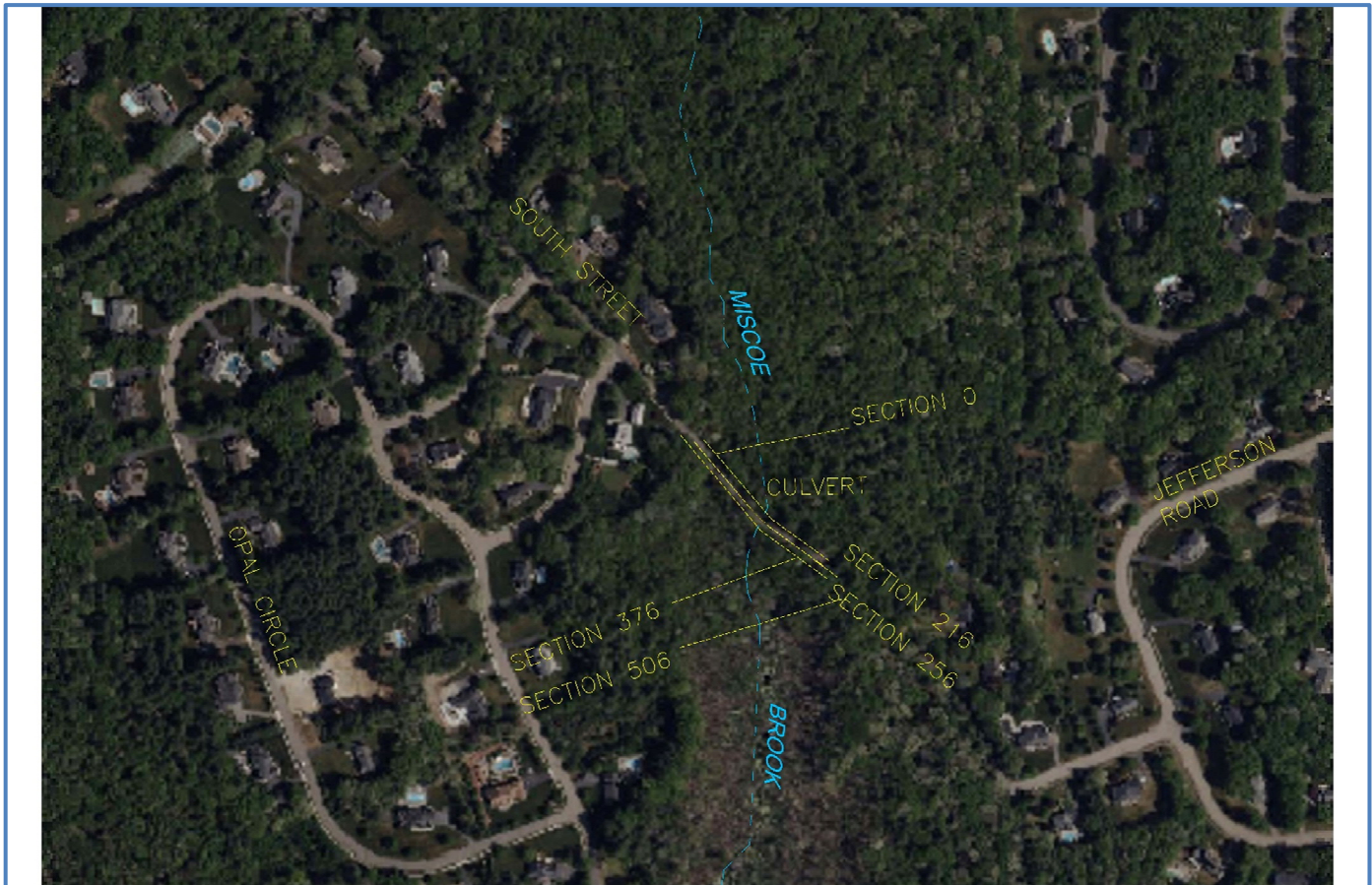
Figure 4-1: HEC-RAS Cross Section Layout Plan
