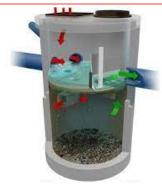
**Leaching Catch Basins** - A leaching catch basin is a pre-cast concrete barrel and riser with an open bottom that permits runoff to infiltrate into the ground.
