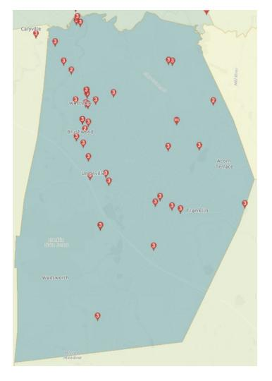
Grade 1: hazardous and must be repaired immediately. This includes leaks in or near a contained space, such as a building or manhole, where the gas could build up enough to potentially explode. Grade 2: non-hazardous, but could become hazardous in the near future Grade 3: non-hazardous and are expected to remain non-hazardous
